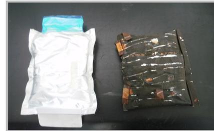
Large battery before and after thermal stability testing in BTC
