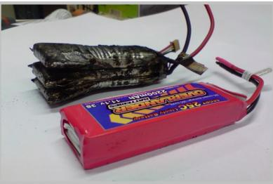
Lithium Polymer batteries after a test in a ‘Standard’ BTC
