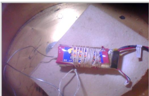
Image during the thermal runaway from the video camera integrated into the BTC
