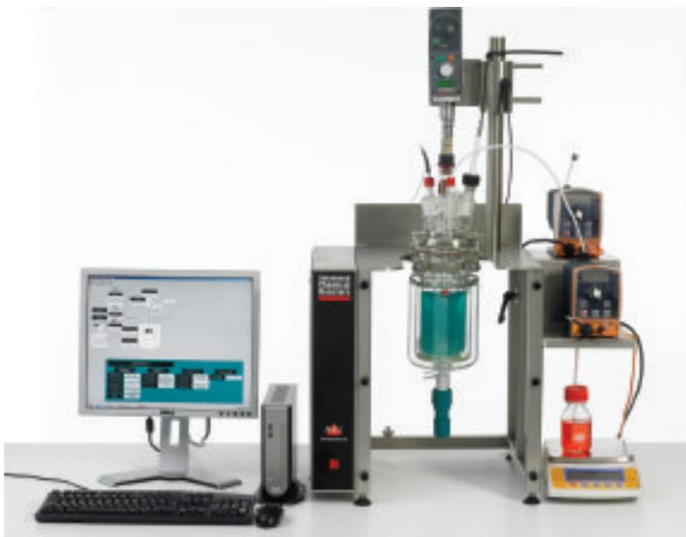
**Figure 3:** Example of reaction calorimeter (SIMULAR)
