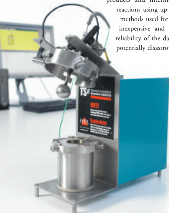
Figure 1: Thermal screening unit (TSU) for screening thermally unstable chemicals
