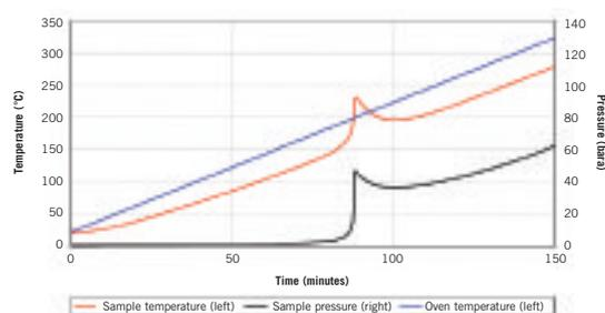
Figure 1: Thermal screening unit (TSU) for screening thermally unstable chemicals
