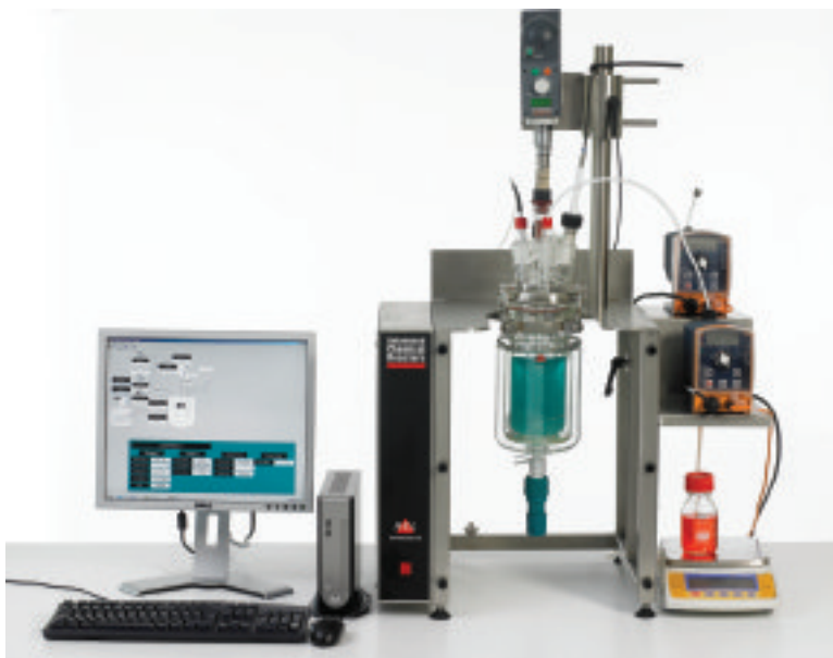
Figure 3: Example of reaction calorimeter (SIMULAR)
