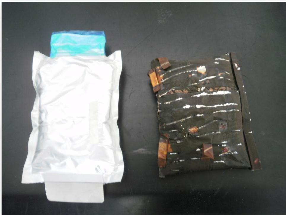
FIGURE 1. LARGE BATTERY BEFORE AND AFTER THERMAL STABILITY TESTING IN BTC
