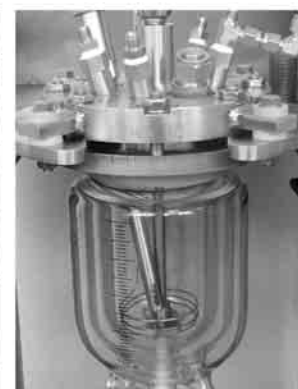
SIMULAR reaction calorimeter (1000 ml)
