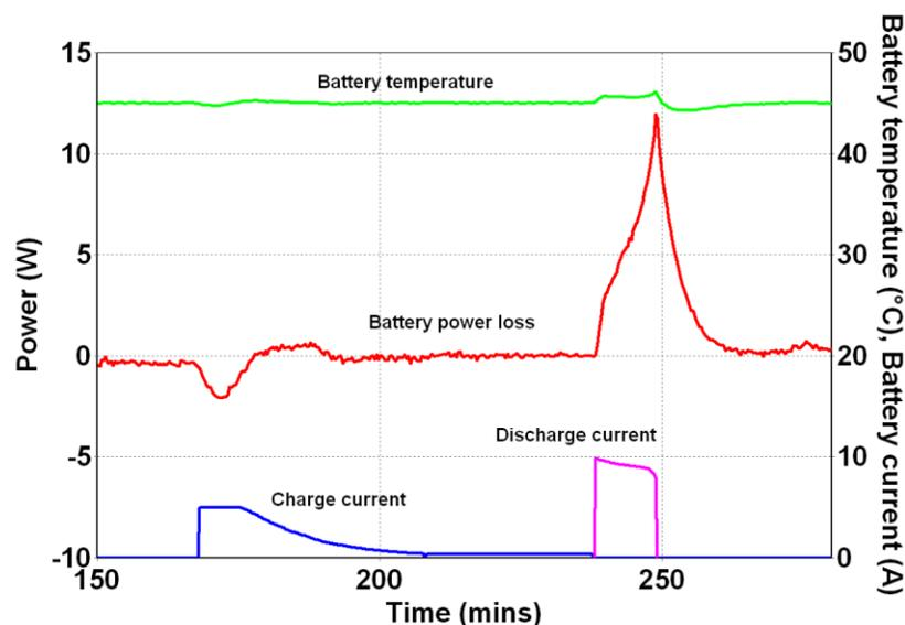
Figure 1: Power Loss (heat output) from Battery during Charge and discharge cycles
