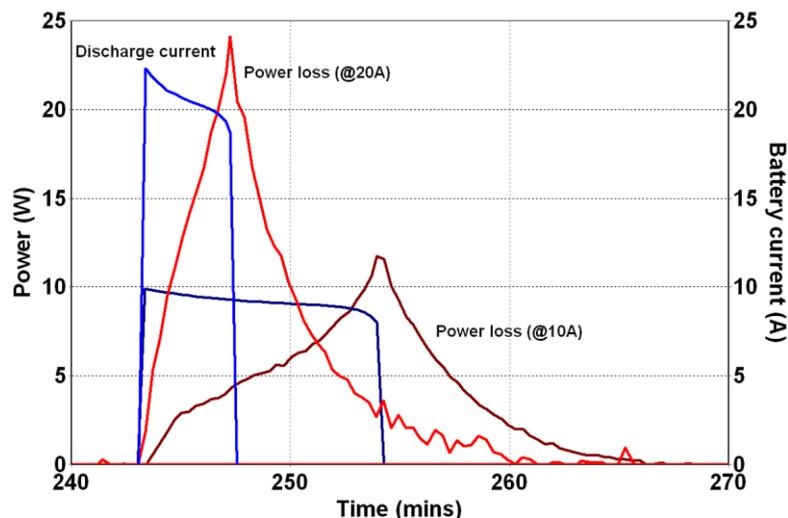
Figure 2: Comparison of battery power loss (heat generation) at different discharge rates
