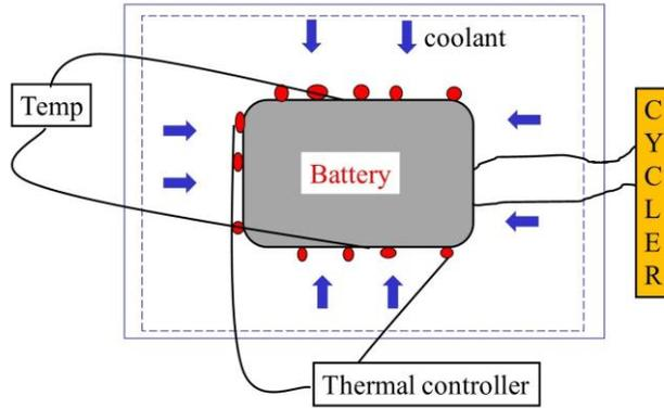
**Figure 3 Working principle of iso-BTC**
